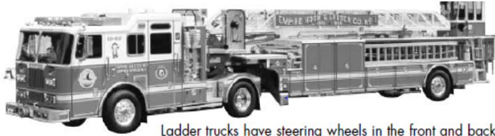
Ladder trucks have steering wheels in the front and back.
